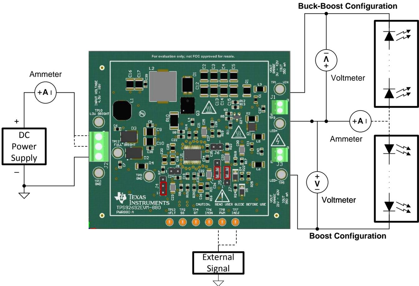
Figure 1. Connection Diagram
