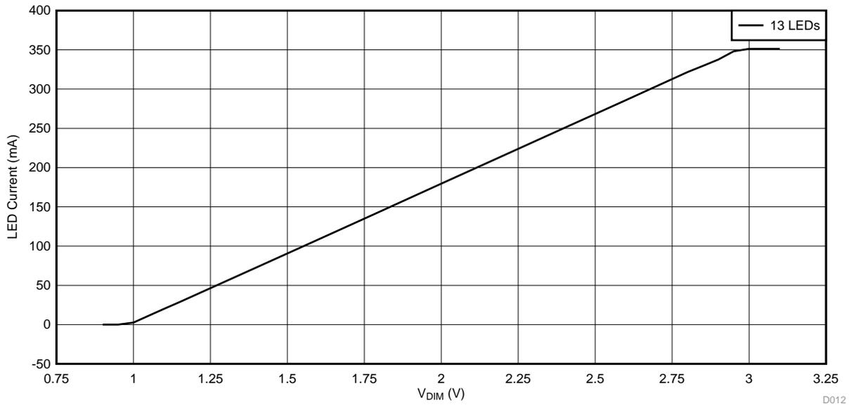
Figure 13. LED Current vs DIM/PWM Voltage ( $V_{IADJ} = 1.49\text{ V}$ , Number of LEDs in Series = 13)
