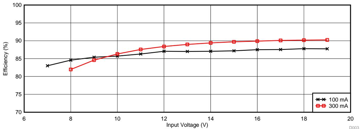
Figure 5. Efficiency vs Input Voltage (Number of Series-Connected LEDs = 18)
