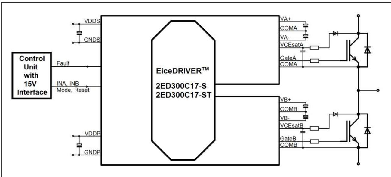
Figure 1: Basic schematic for driver setup
