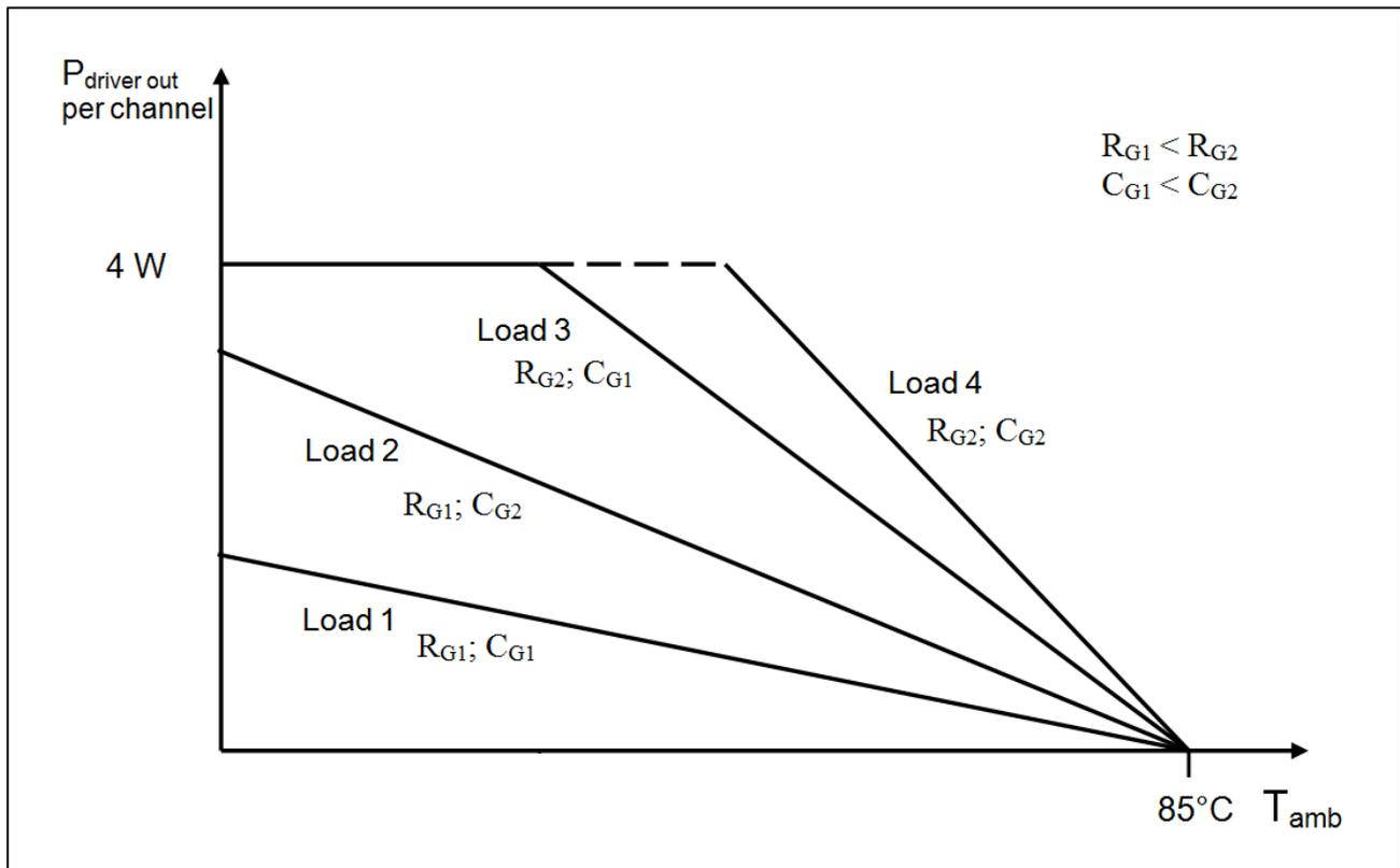
Figure 6: Power dissipation of the driver for different load conditions
