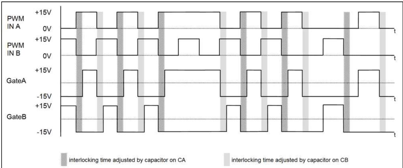
Figure 8: PWM timing diagram with interlocking time functionality
