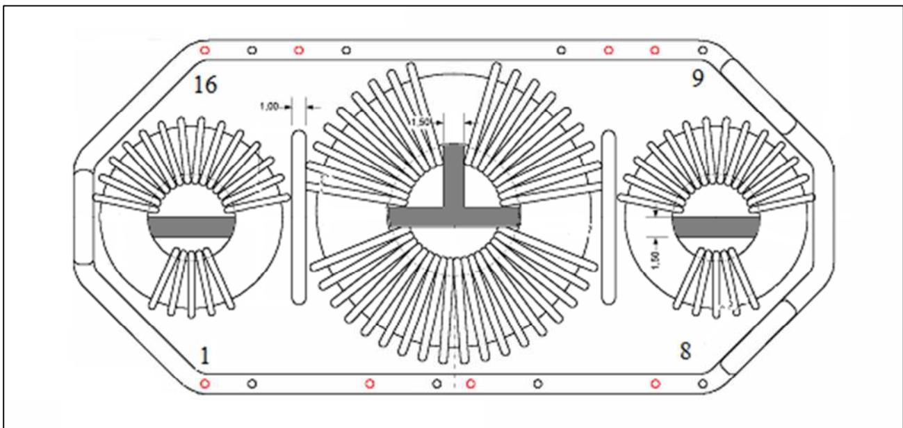
**Figure 4: Additionally mechanical barriers for high isolation solution**
