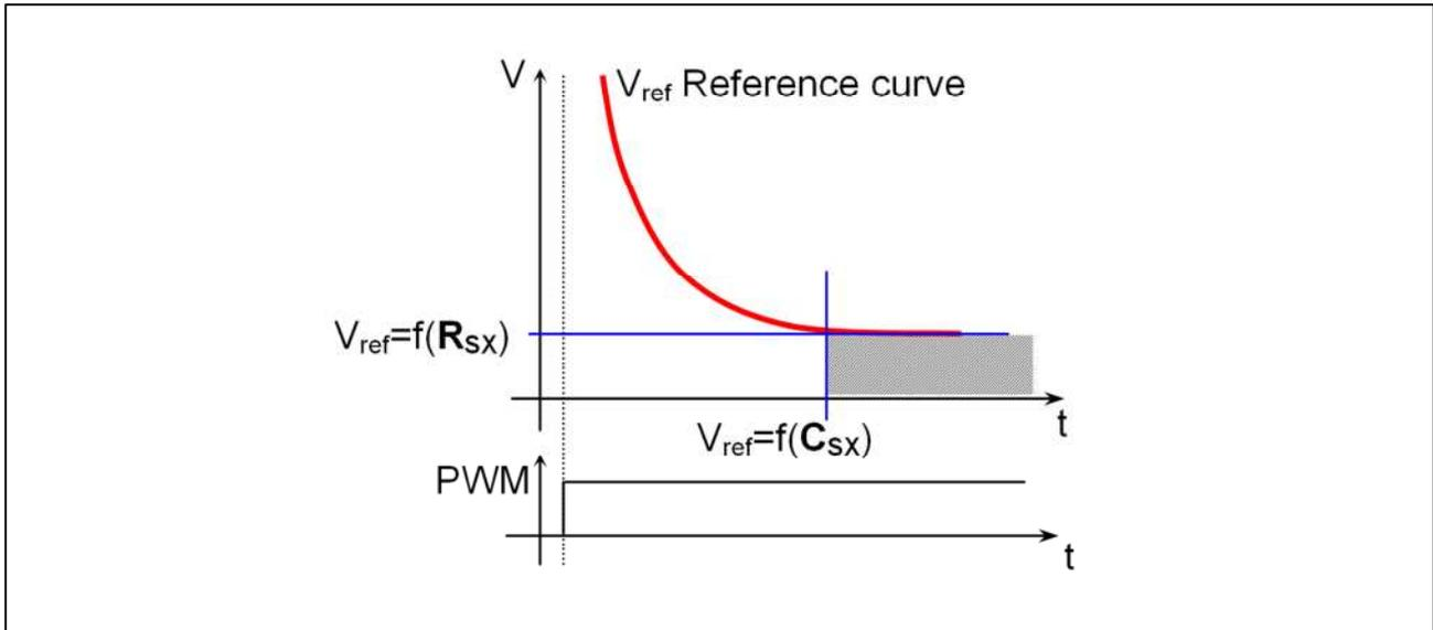
**Figure 7: Vce,sat reference curve**
